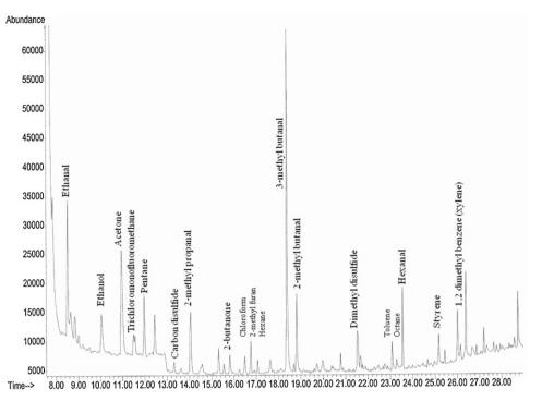
Fig. 2. GC/MS chromatogram showing the soil headspace analysis collected from an 11 year-old shallow grave in sandy soil indicating relevant compounds commonly seen using odor mortis as a means of locating human clandestine graves.
