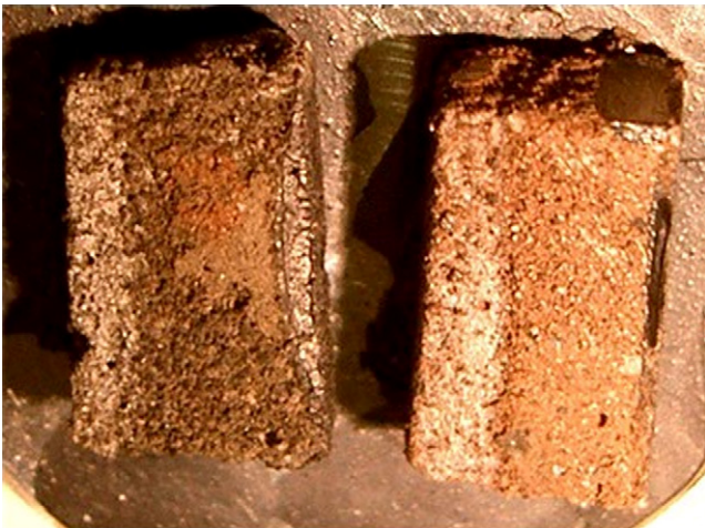
Fig. 7. Photograph of two samples exposed to vacuum for 60 days. (Left) Sulfur ~35 wt% JSC-1. (Right) Sulfur ~55 wt% JSC-1 ~20 wt% SiO 2 .
