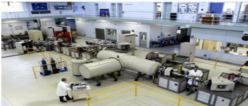
Figure.3: Accelerator mass spectrometer
