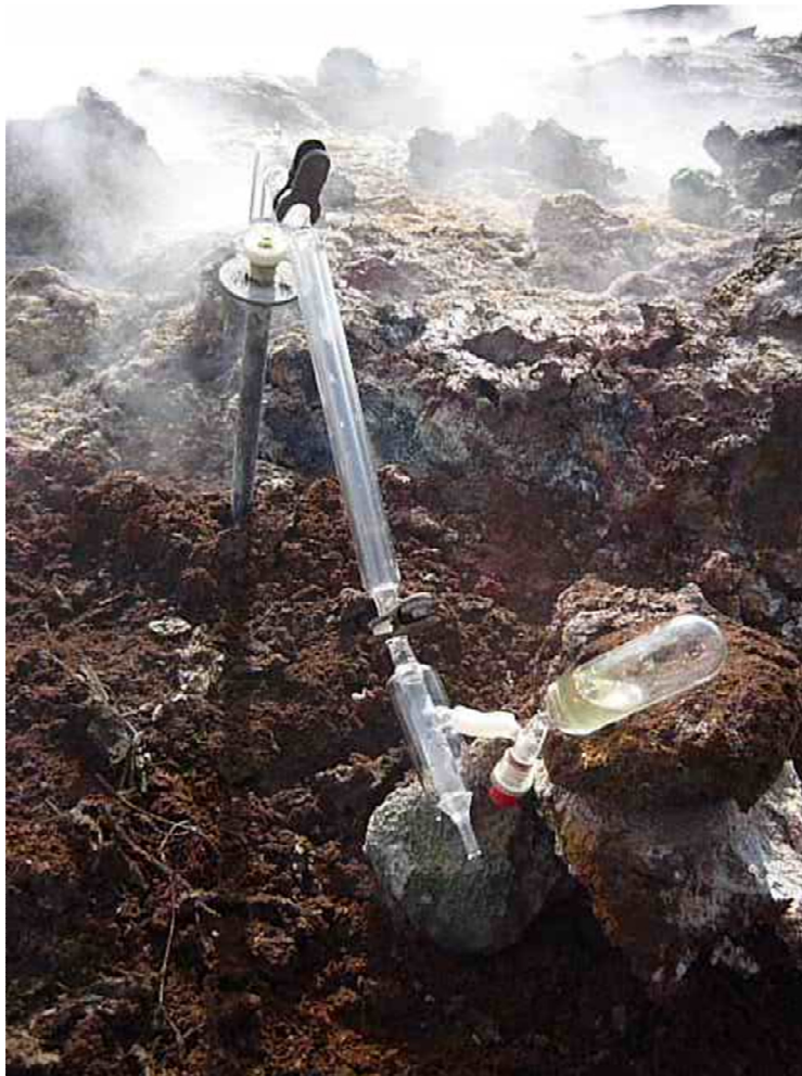
Figure 2.1.3.: Gas sampling line for fumaroles.
