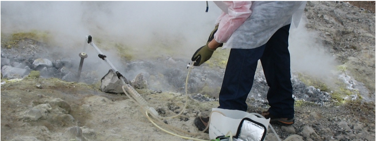
Figure 2.1.4.: Sampling line for VOCs using water/ice-cooled glass device (Graham type condenser).
