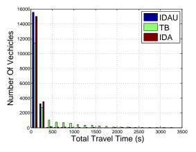
Fig. 6: Travel time distributions for a flow rate of 8000veh/h.
