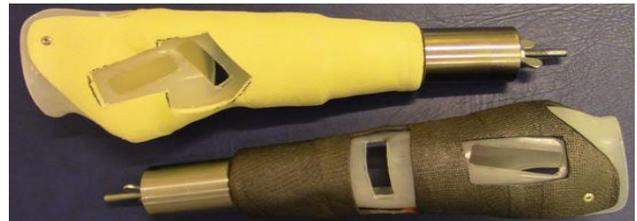
Fig. 1. Two custom made test sockets. The features of them are the same as the daily used sockets in combination with a prosthetic hand (Michelangelo hand, Otto Bock Healthcare Products GmbH).
