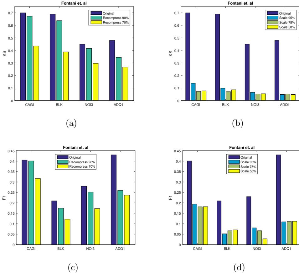
Figure 13: Evaluation of robustness on the Fontani et al. dataset: a-b) KS scores on the original dataset and after recompressions -rescales, c-d) F1 scores on the original dataset and after recompressions -rescales.
