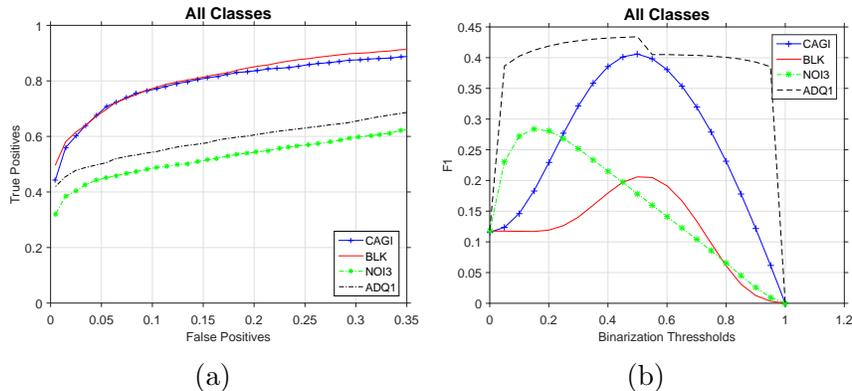
Figure 8: Results in the Fontani et al. synthetic dataset over all classes: a) ROC curves, b) F1 score curves.
