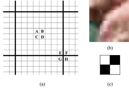
Figure 1: a) Depiction of JPEG  $8 \times 8$  grid (bold lines) over image pixels. Pixels labeled A-D are sampled periodically to represent the inner part of the grid, while E-H are sampled on grid intersections [3], b) 32x32 JPEG image displaying visible grid artifacts, c) Pixel intensity pattern (cross pattern) maximizing  $Z'$  and  $Z''$  (Equation 1).
