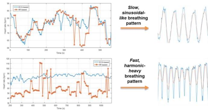
Fig. 8: ECG-based (blue) and RF-based (orange) HR estimation during sinusoidal (top) and fast, harmonic-heavy (bottom) respiration
