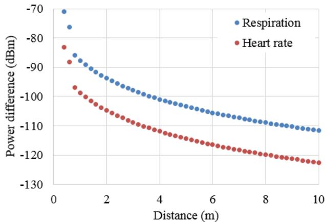
Fig. 5: Expected Rx power difference over distance for human target sitting in front of the radar due to HR and BR
