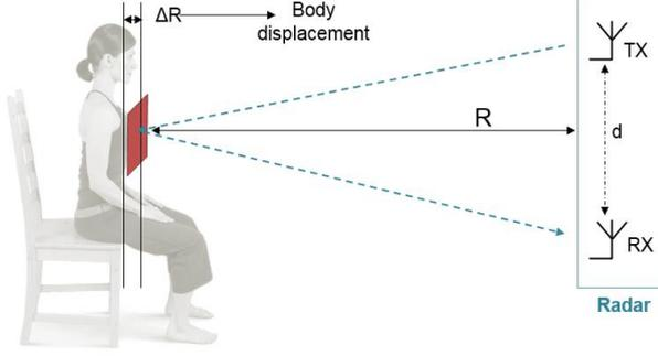
Fig. 3: Measurement principle of VS with the radar-based sensor
