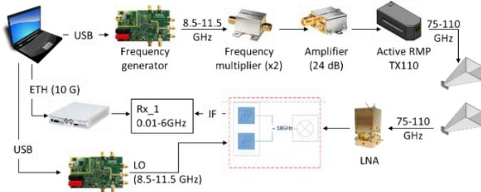
Fig. 1: The VSM system detail block diagram.
