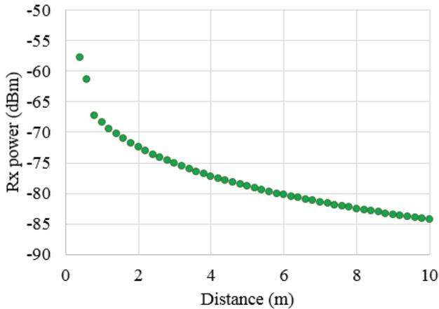
Fig. 4: Expected Rx power over distance for human target sitting in front of the radar
