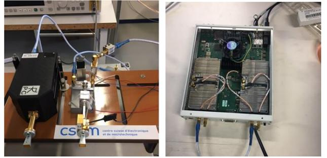
Fig. 2: Over view of the VSM system, RF-front-end (a) and SDR based platform (USRP X310) (b).
