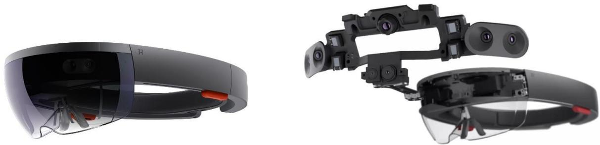
Fig2: Assembled and disassembled views of the HoloLens MR device.
