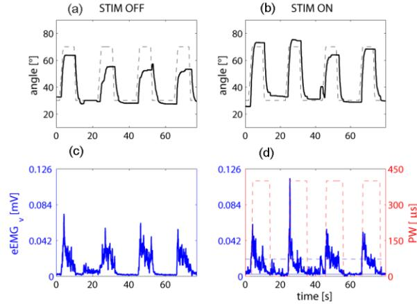
**Figure 4.** Tracking performance of an individual with SCI during elbow flexion without and with FES. The ON/OFF controller was used to modulate the pulse width (PW). Panels a-b: measured (solid line) and target angle (dashed line); panel c: volitional EMG; panel d: volitional EMG (blue), PW (red); ON/OFF thresholds (horizontal lines).
