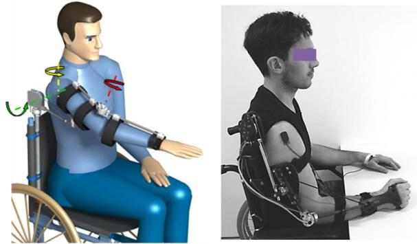
**Figure 1.** The 3-DOF exoskeleton arm for weight relief.
