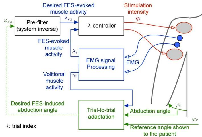
Figure 3. Control scheme of the “assist-as-needed” controller.
