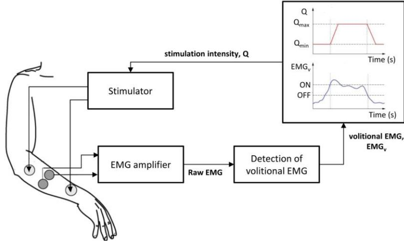
**Figure 2.** Control scheme of the ON/OFF controller.
