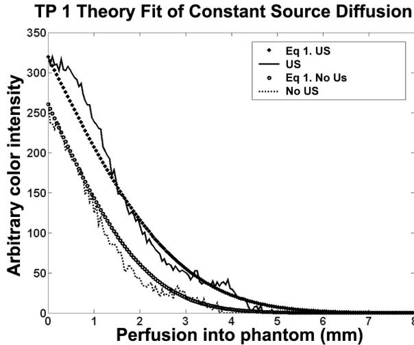
Fig. 3. Plot of the theoretical fit to the experimental data for TP 1. We see good agreement with control (No US) and the constant source diffusion Eq. (1), note that US experimental data does not fit Eq. (1) well.
