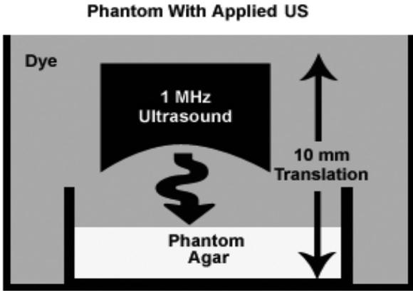
Fig. 1. The experimental setup for the phantom study is shown. The sonicated phantom is immersed in 0.5 wt% diluted dye and pulse sonicated (15 seconds on and off) while simultaneously the transducer is oscillated up and down at 0.25Hz 10mm amplitude. The beginning position of the transducer was 40mm above the agar/dye interface, so that the US focus was placed on the surface. The control setup was the same without US.
