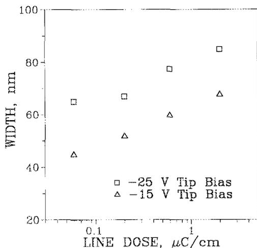
FIG. 3. Developed linewidth vs line dose for STM lithography in SAL-601
