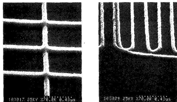
FIG. 2. STM written patterns in SAL-601 which have been transferred into the GaAs substrate by RIE. The left pattern was written at  $-35$  V and 60 nC/cm. The right pattern was written with the same dose at  $-15$  V, also at 60 nC/cm.
