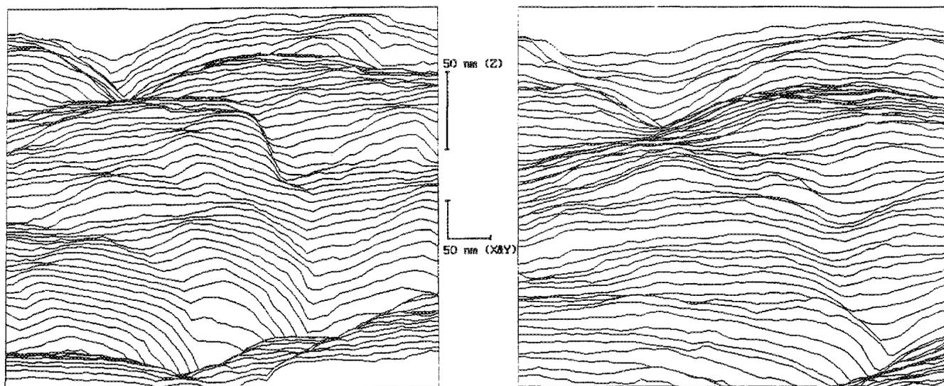
FIG. 4. The same surface imaged with the STM under tunneling,  $-0.6$  V tip bias (left) and field emission,  $-35$  V tip bias (right).
