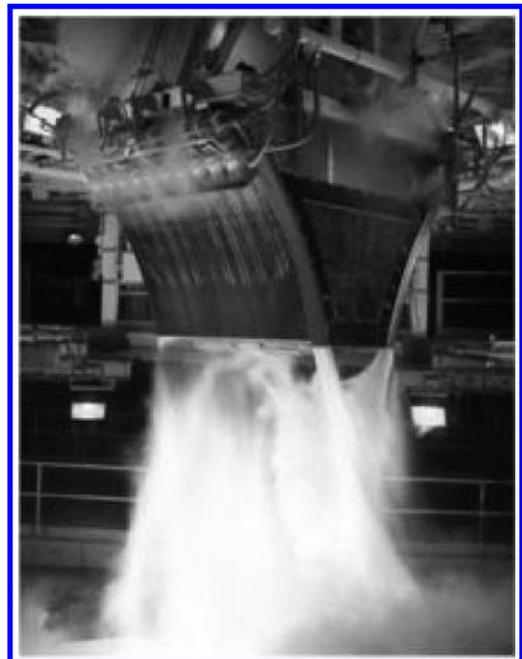
**Fig. 12 XRS-2200 aerospace engine.**
