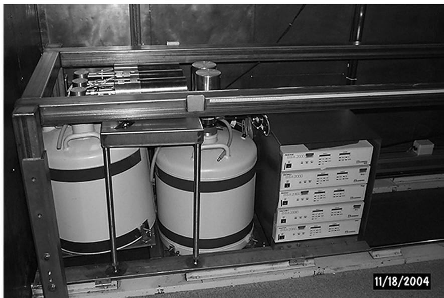
Figure 1. Coaxial germanium measurement system.
