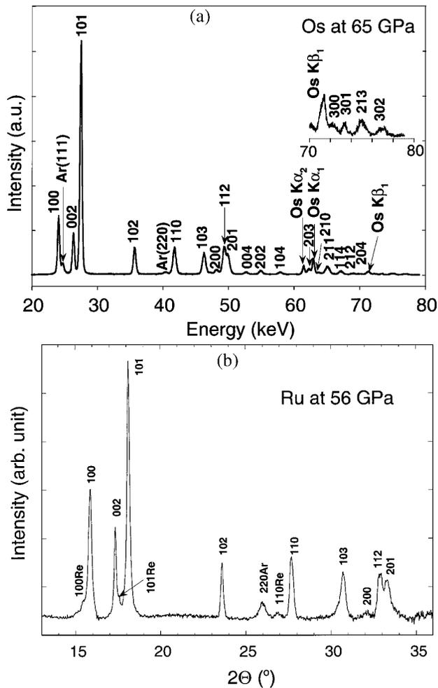
FIG. 1. Energy-dispersive x-ray diffraction pattern for hcp Os at 65 GPa in (a). Inset shows an expanded view from 70 to 80 keV. Angle-dispersive x-ray diffraction pattern for hcp Ru at 56 GPa in (b). The Ar and Re peaks are marked. The refined result for the lattice constants of Os is  $a = 2.5907 (\pm 0.0014) \text{ \AA}$  and  $c = 4.1161 (\pm 0.0017) \text{ \AA}$ .
