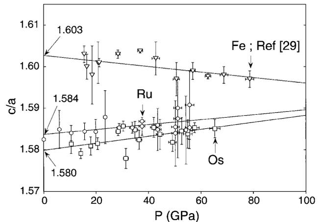
FIG. 3. Plot of experimentally measured  $c/a$  ratios for Fe (inverted triangles) [29], Ru (open circles), and Os (open squares) at high pressures and including error bars. The solid lines are linear fits to the data and are shown as guides to the eye.
