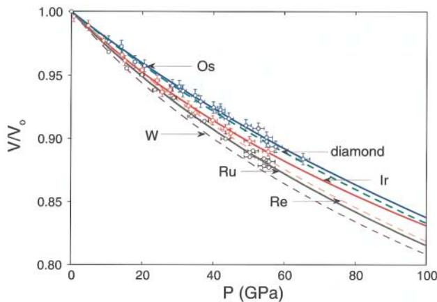
FIG. 2 (color). Volume compressions for Os, Ir, Re, Ru, W, and C. Previously measured Re (orange dashed line) [21], W (purple dashed line) [22], and diamond (green dashed line) [4] data were included for comparison. Error bars are shown for Os, Ir, and Ru.
