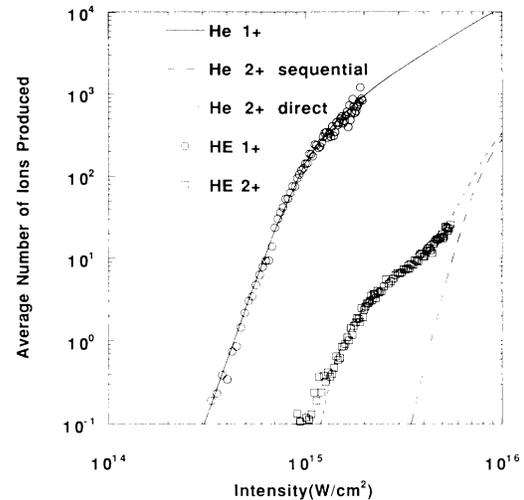
FIG. 3. Ion yield data compared to sequential and nonsequential numerical solution of the Schrödinger wave equation. The data for both charge states have been uniformly shifted down in intensity by a factor of 1.25 for comparison with theory.
