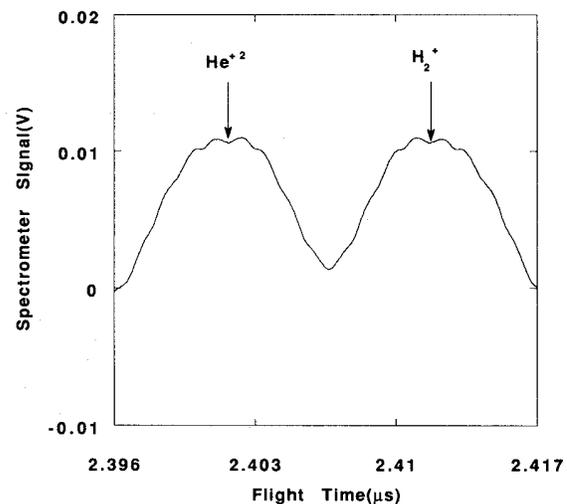
FIG. 1. Resolution of He<sup>+2</sup> and H<sub>2</sub><sup>+</sup> ions.
