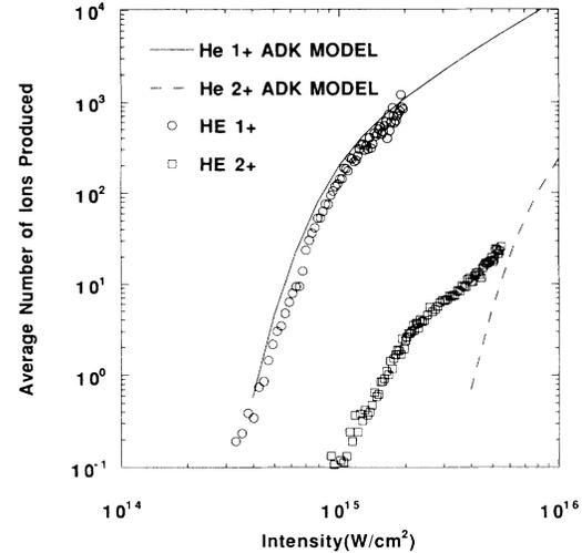
FIG. 2. Ion yield data compared to sequential ADK theory. The data for both charge states have been uniformly shifted down in intensity by a factor of 1.25 for comparison with theory.
