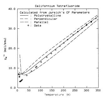
FIG. 2. Experimental and calculated inverse magnetic susceptibility of  $CfF_4$  vs temperature.
