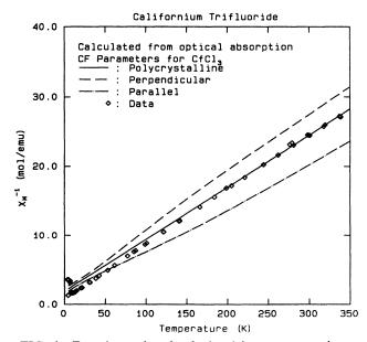
FIG. 1. Experimental and calculated inverse magnetic susceptibility of  $CfF_3$  (orthorhombic) vs temperature.
