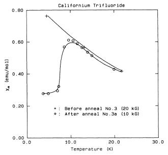
FIG. 3. Magnetic susceptibility of polycrystalline  $CfF_3$  (or-thorhombic) at low temperatures.
