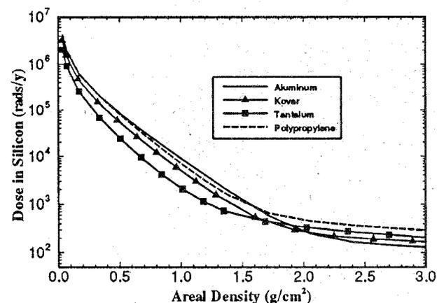
Fig. 3 Dose-vs-depth for omnidirectional natural trapped electrons at 20,175-km, 55°-inclination, circular orbit for single-material slab shields.
