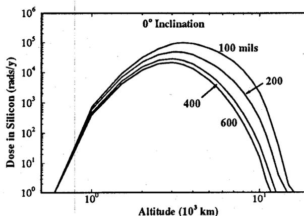
Fig. 2. Natural trapped proton dose in silicon versus altitude for slab aluminum shields of various thicknesses.
