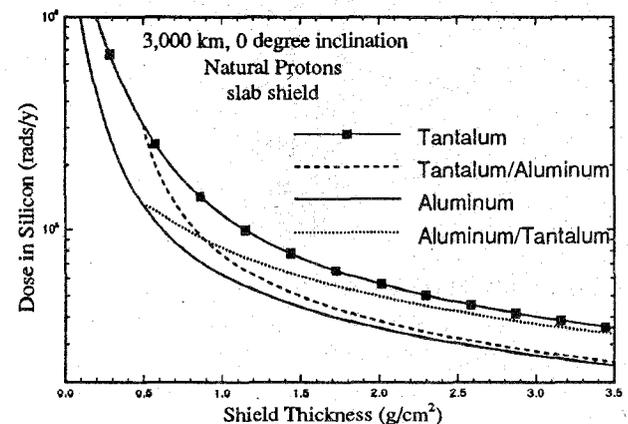
Fig. 7 Comparison of single-material and multi-layer shield effectiveness for natural trapped protons.
