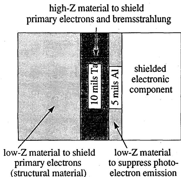
Fig. 4 Schematic of a three-layer shield design.
