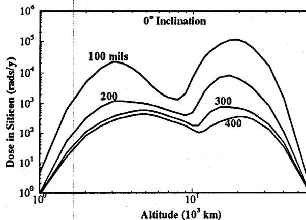
Fig. 1 Natural trapped electron dose in silicon versus altitude for slab aluminum shields of various thicknesses.
