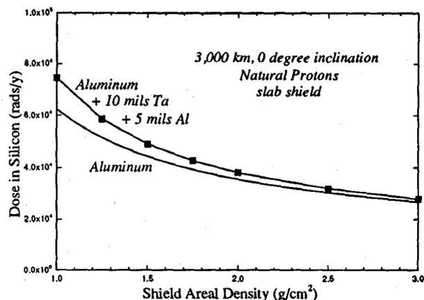
Fig. 8 Comparison of single-material and three-layer shield effectiveness for natural trapped protons.
