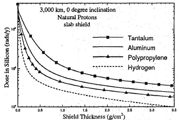
Fig. 6 Dose-vs-depth for natural trapped protons at 3,000 km,  $0^\circ$  inclination.
