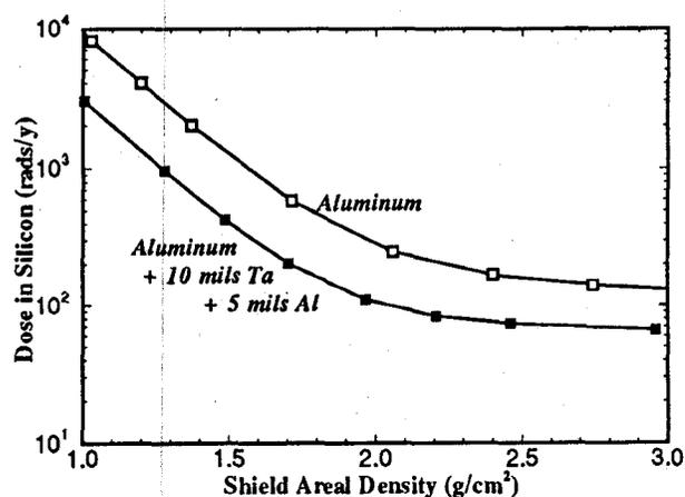
Fig. 5 Slab shield dose-vs-depth comparison for omnidirectional natural trapped electrons at 20,175-km, 55°-inclination, circular orbit.
