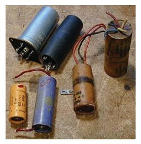
Figure 3. Examples of early electrolytic capacitors taken from antique radios. These capacitors are also unreliable and are replaced when restoring such a radio. Photo courtesy of P. I. Nelson, www.antiqueradio.org, and used with permission.
