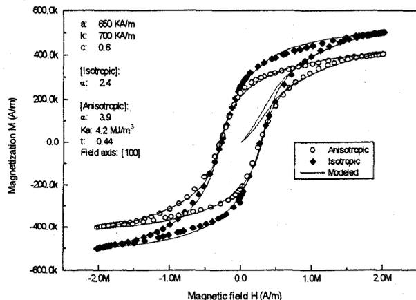
Fig. 3. Modeled and measured hysteresis curves of sample 3 without heat treatment
