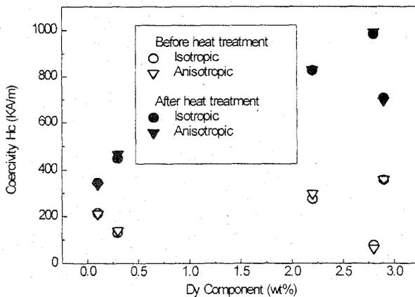
Fig. 1. Measured coercivities  $H_c$  of NdFeB materials versus Dy component.
