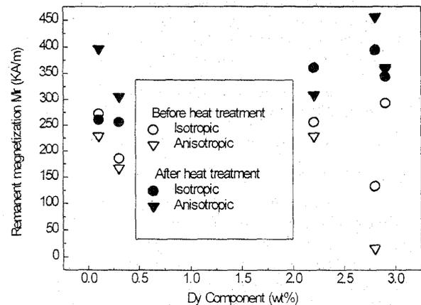
Fig. 2. Measured remanent magnetization  $M_r$  of NdFeB materials versus Dy component.
