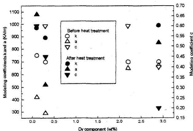
Fig. 5. Modeling coefficient versus Dy component of NdFeB materials
