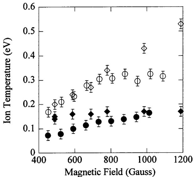
FIG. 2. ( $\diamond$ ) Perpendicular and ( $\blacklozenge$ ) parallel ion temperature measurements as a function of magnetic field strength in HELIXa for a fill pressure of 2 mTorr, a rf driving frequency of 9 MHz and a rf power of 400 W. ( $\circ$ ) Perpendicular and ( $\bullet$ ) parallel ion temperature measurements as a function of magnetic field strength in HELIXb for a fill pressure of 6.7 mTorr, a rf driving frequency of 9 MHz and a rf power of 750 W.
