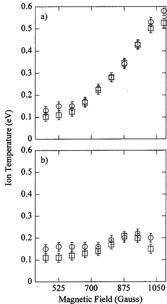
FIG. 3. (a) On axis ( $\circ$ ) perpendicular and ( $\square$ ) parallel ion temperature as a function of magnetic field strength for HELIXb in the eight-coil configuration at position "B" with a fill pressure of 6.7 mTorr, and 750 W of rf power for (a) a rf frequency of 9 MHz and (b) a rf frequency of 13.5 MHz.
