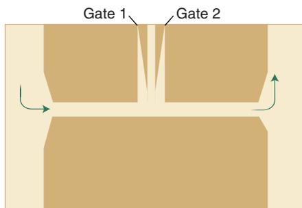
**Creating a spin current through spin pumping I.** A single channel of electrons is formed in a 2D electron system through electrostatic confinement. When out-of-phase ac voltages are applied to the two gates, the channel is perturbed, resulting in a dc electron current. If one of the gates is replaced by an oscillating magnetic field, a spin current is pumped.
