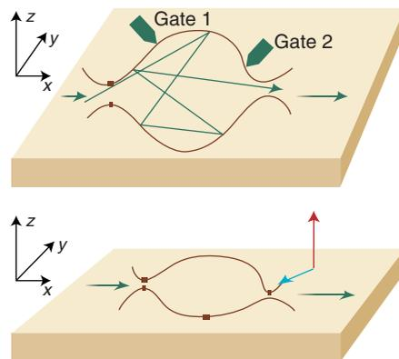
**Creating a spin current through spin pumping II.** (Top) A quantum cavity is perturbed through out-of-phase ac voltages applied to the two gates. Electrons entering the cavity scatter off the cavity walls several times before leaving. (Bottom) In a sufficiently large cavity, pumping leads to a spin current with a tunable direction of spin polarization. Both in-plane (green arrow) and out-of-plane (red arrow) polarizations are possible.
