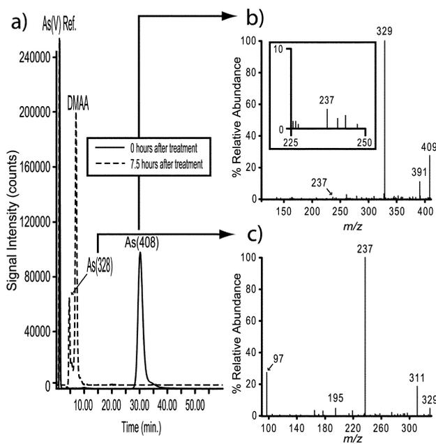
**Fig. 3** Degradation of As(408) in time using IC-ICP-MS and IC-ESI-MS for structural verification. (a) IC-ICP-MS chromatogram of As(408) in 2.5% TMAOH at 0 h (solid line) and 7.5 h after treatment (dashed line) at 60 °C. (b) ESI-MS/MS spectra of starting arsenosugar, As(408). (c) ESI-MS/MS spectra of degradation product, As(328).
