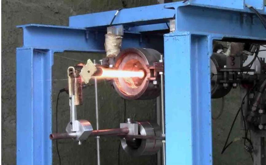
Figure 34 Preliminary Configuration Free jet test at Aerospace Propulsion Laboratory of University of Naples "Federico II".
