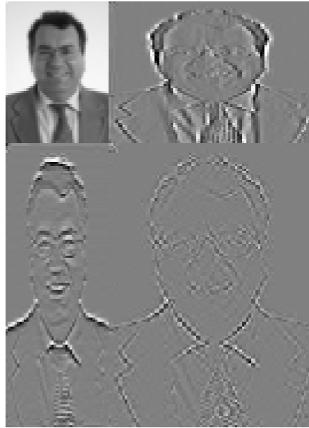
Figure 8. 2D unbalanced lifting wavelet transformed image with p=3:1 and q=3:2 . Highband subimages are amplified by a factor of three.
