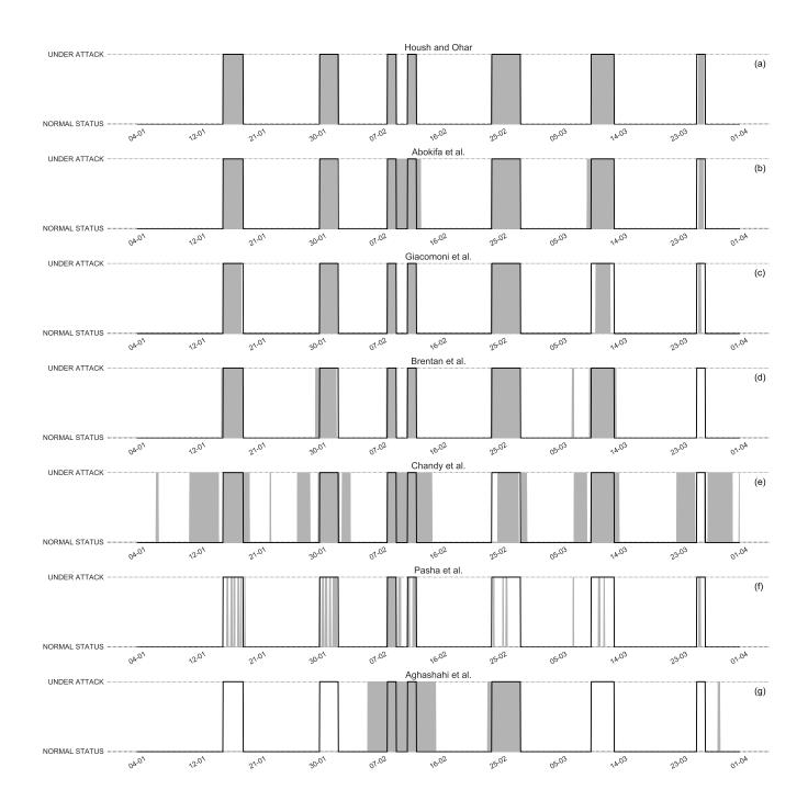
FIG. 4. Comparison between actual and detected attacks (gray area and black line, respectively) for the *Test dataset*. Each panel corresponds to a different attack detection algorithm.
