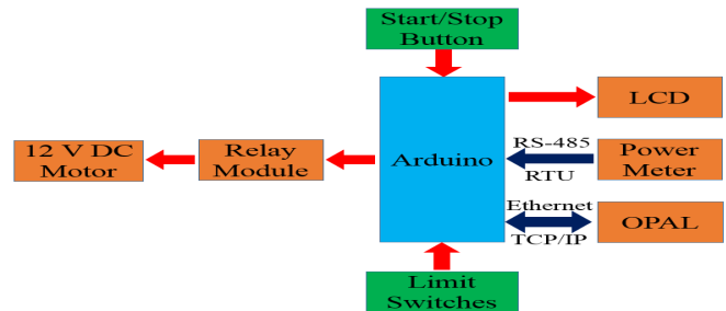
Fig. 2 – Controlling process of the 4 kVA load.
