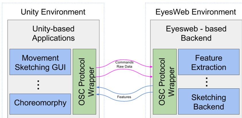
Figure 6. Unity Integration schema and communication protocol between Unity-based and Eyesweb-based applications
