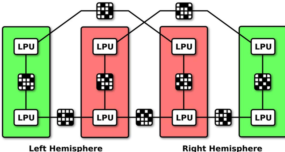
Figure 4: Hierarchy of modeling components in a Neurokernel fly brain model. LPUs and connectivity patterns may be composed into subsystems (red, green) which may in turn be connected to other subsystems.
