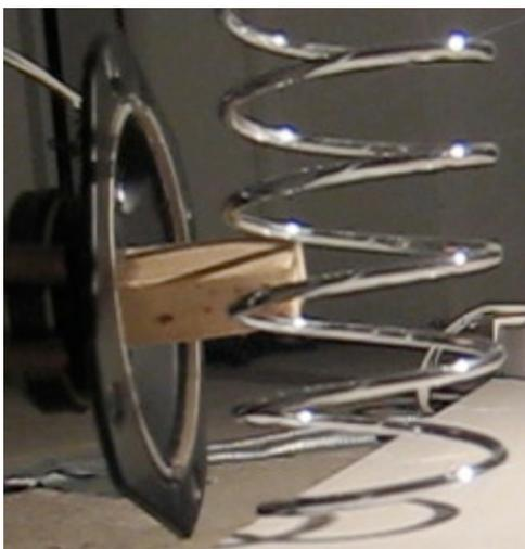
Figure 3. Prepared speaker vibrating spring
