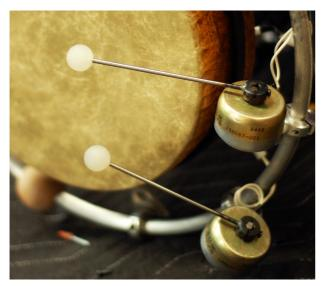
Figure 2. TrimpTron Solenoids
