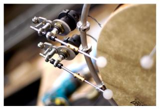
Figure 3. KalTrons on the NotomotoN's Superstructure
