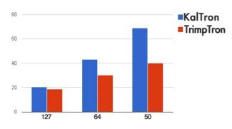
Figure 5. Actuator Speed Tests (X-axis = MIDI velocity; Yaxis = Strikes/Second)
