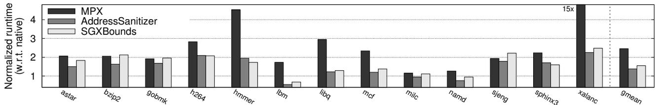
Figure 12: SPEC outside of SGX enclave (normal unconstrained environment): Performance overhead over native execution.
