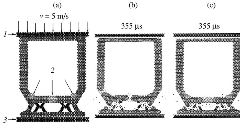
**Fig. 1.** Schematic diagrams (a) of the base model construction and the patterns of fracture in the frame (b) with and (c) without damping inserts at the time moment  $t = 355 \mu\text{s}$ : (1) piston; (2) damping inserts; (3) immobile obstacle.
