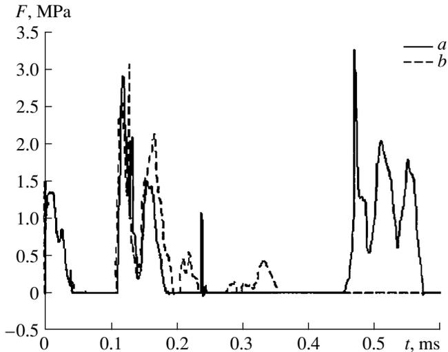
**Fig. 3.** Time variation of the response force acting upon the "piston" for the frame structures with crosspiece in different positions (curves *a* and *b* correspond to variants of the same notation in Fig. 2).
