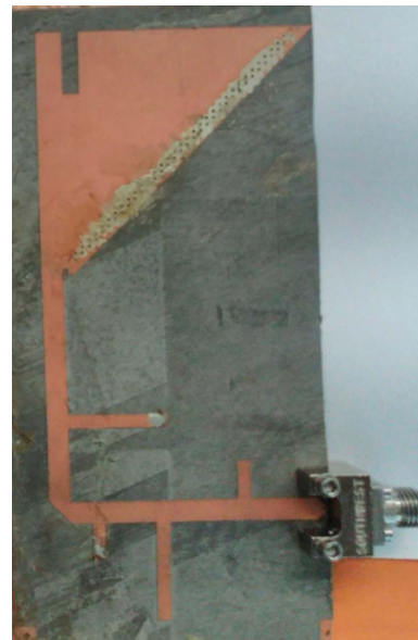
Fig. 5. Prototype dual band antenna that operates in 2.4GHz and 5GHz.
