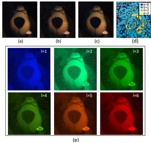
Fig. 5. Simulation results data cube 3 (a) RGB mapping original scene; (b) RGB mapping of the full-resolution reconstruction; (c) RGB mapping of the proposed reconstruction; (d) Blocks of pixels from proposed approach; (e) Recovered spectral bands.
