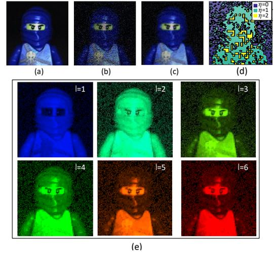
Fig. 3. Simulation results data cube 1 (a) RGB mapping original scene; (b) RGB mapping of the full-resolution reconstruction; (c) RGB mapping of the proposed reconstruction; (d) Blocks of pixels from proposed approach; (e) Recovered spectral bands.
