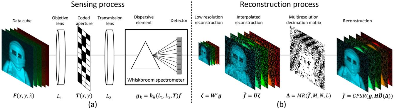
Fig. 1. (a) Single pixel camera (SPC) sensing and (b) Proposed multi-resolution (MR) reconstruction process.
