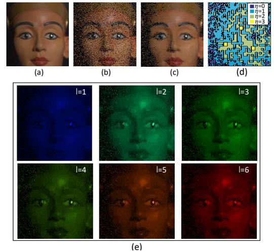
Fig. 4. Simulation results data cube 2 (a) RGB mapping original scene; (b) RGB mapping of the full-resolution reconstruction; (c) RGB mapping of the proposed reconstruction; (d) Blocks of pixels from proposed approach; (e) Recovered spectral bands.
