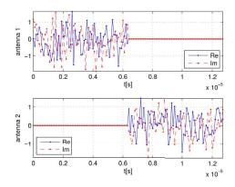
Fig. 2. Time domain signals in each of the two available antenna ( $N_T=2$ ) for a configuration with bandwidth of 10 MHz and 128 subcarriers.
