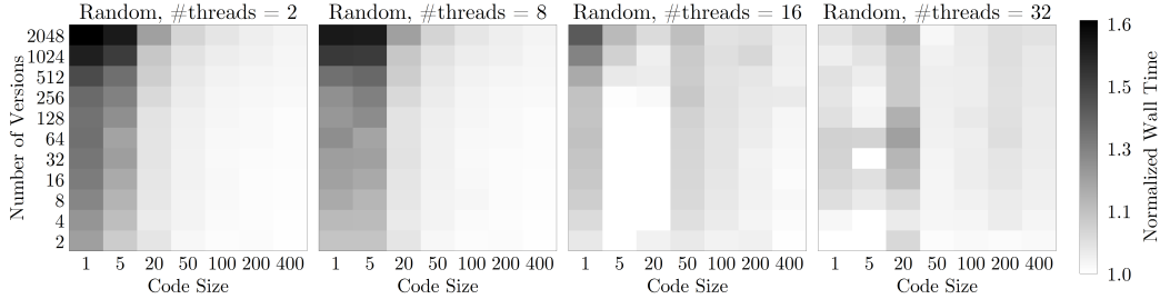
Figure 5: PowerPC system normalized wall time, two inner iterations, across varying numbers of threads.
