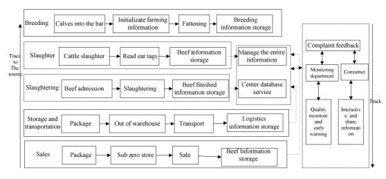
Figure 1. Quality beef traceability system architecture and data flow
