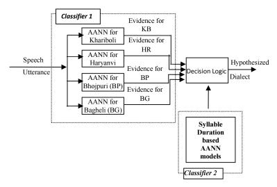
Figure 5. Block diagram of dialect identification system based on evidences from each dialect
