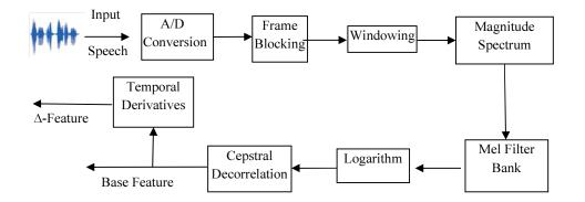
Figure 1. Block diagram of Mel frequency cepstral coefficients
