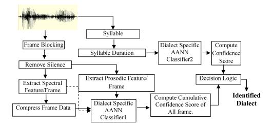
Figure 4. Flow graph of AANN based dialect identification system
