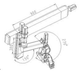
Figure 4. Motion range of robot arm
