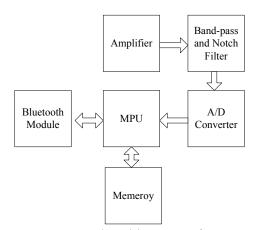
Figure 7. Conceptual architecture of ECG module
