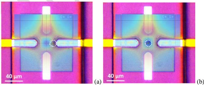
Fig. 2. Comparison of electric field intensity distribution on the quadrupole electrode structure (red high intensity, blue low intensity) and the optimal cell electrical trap region in (a) positive DEP and (b) negative DEP cases.
