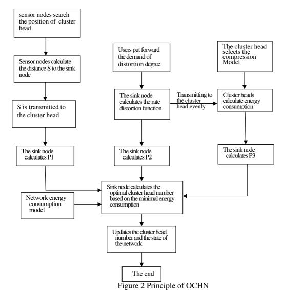
Step 1: the sink calculates the radius of each cluster according to the area radius and the initial cluster  $k_0$ , and transmits the result to all of sensor nodes.
