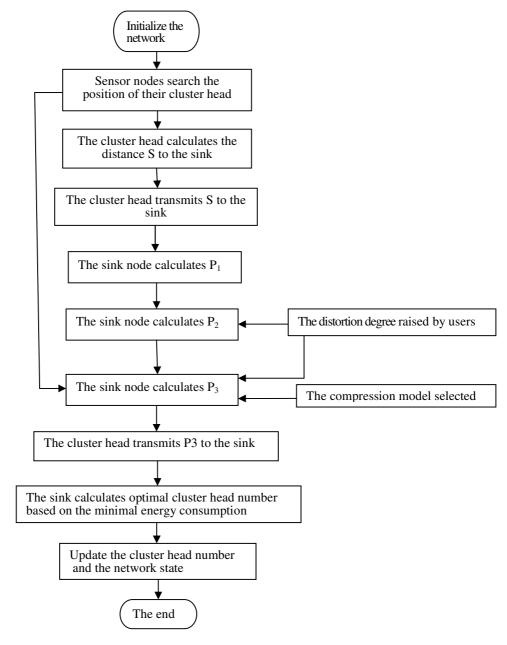
Figure 3. Process flow of OCHN
