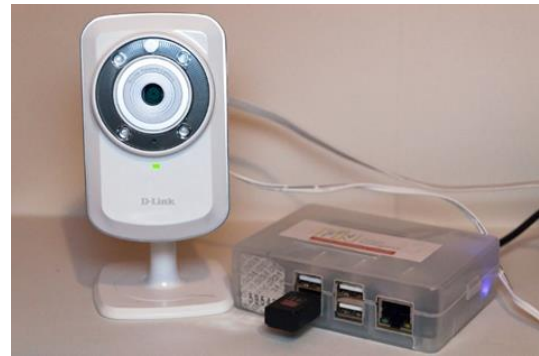
Fig. 2. FINT Ltd. embedded system prototype with network camera.
