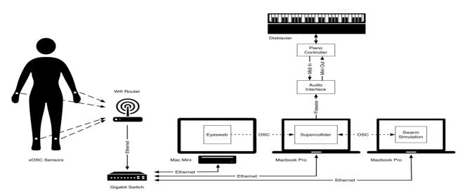
Figure 5-2. Schematic Depiction of Technical Integration of the Sensing, Communication, Computation and Piano Control
