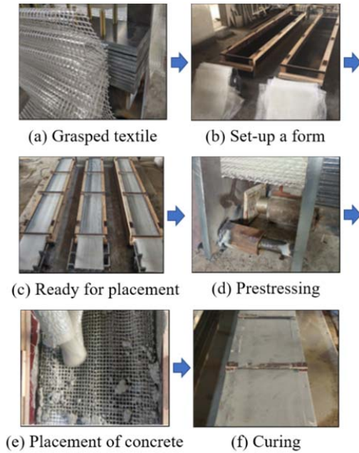
Fig. 3 Manufacturing procedure of TRC specimen
