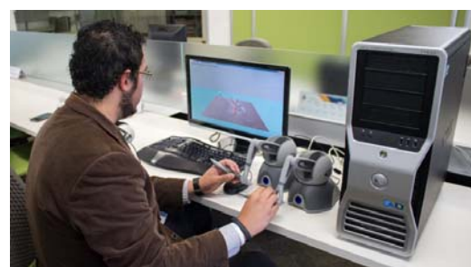
Fig. 8 User interacting with a mechanical visuo-haptic environment using virtual prototyping and app development platforms
