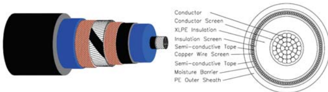
Fig. 3 Single core submarine power cable cross section [3]
