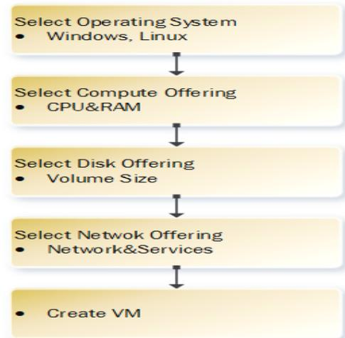
Fig. 3 Virtual Machine Instance Creation Steps
