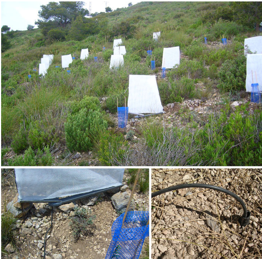
Fig. 7 Top: General view of the experimental fog collection plot established in Crevillente (SE Spain). Bottom: details of the channel (left) and micropipe (right) to carry the collected water towards the seedling root zone
