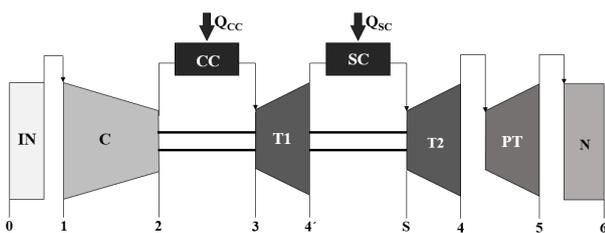
Fig. 2 Diagram of the modified turboshaft configuration
