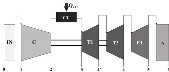
Fig. 1 Diagram of the reference turboshaft configuration
